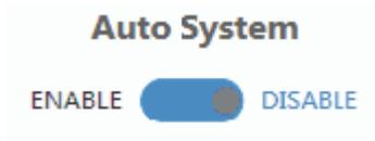
**Auto System:** When the toggle is in ‘enable’ position and the system is in standby status, if a new signal is connected, the system will change to active and fully controllable. When the toggle is in ‘disable’ position and the system is in standby status, if a new signal is connected, the system status won’t change.
