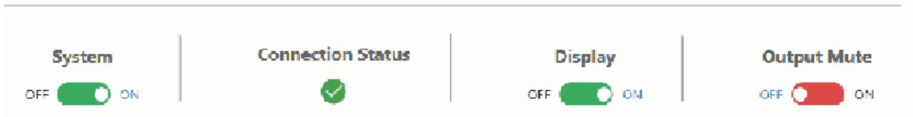
**System** – runs the system on/off subroutine when switches the toggle. (see section 7)
