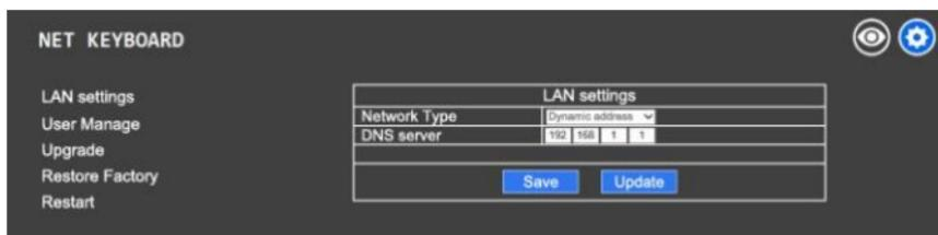
Dynamic address (default access method): the keyboard will automatically request an IP address from the router.
