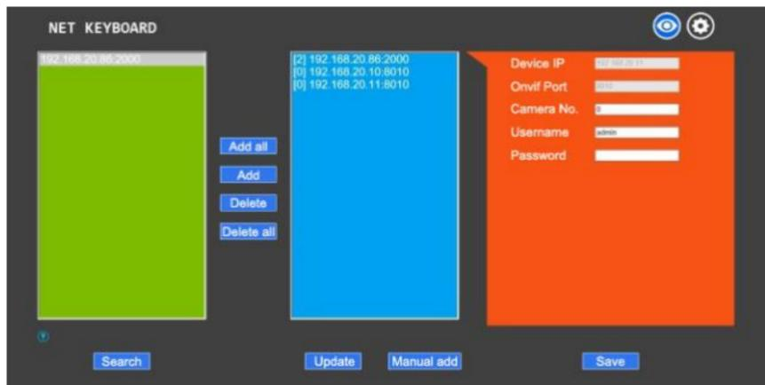
4. After entering the device home page, the three lists are: search device list (green box); device list (blue box) added; device details (orange frame); manual addition (yellow box).
