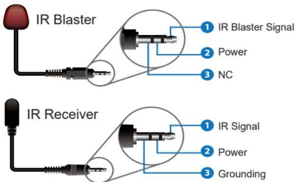
*Note: IR remote sends signal at the distance of 0~5 meters / 0~8 meters with the angle of  $\pm 45^\circ$  in vertical direction.*
