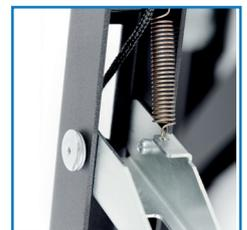
Adjusting the retractable mechanism spring provides quick and easy access for servicing.
