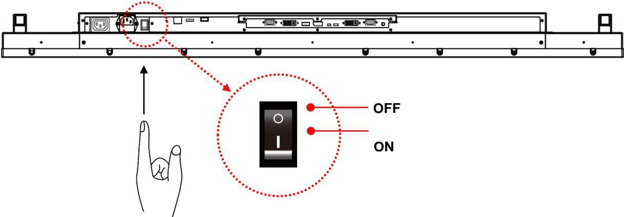
**NOTE:** The remote control only works when the power switch is ON.
