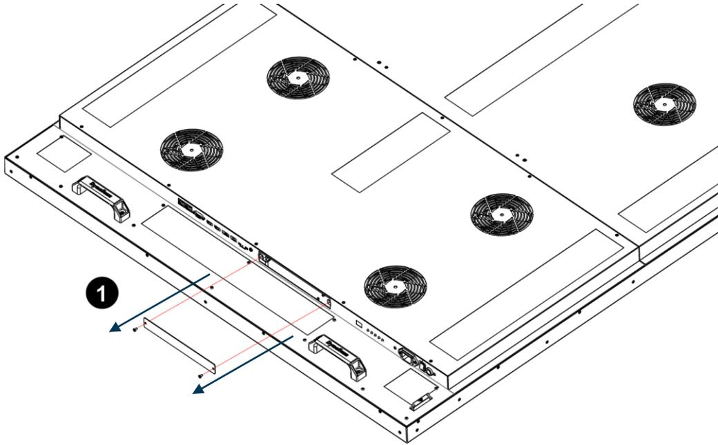
2. Insert the SDM module into the display and fasten screws. Make sure the SDM properly installed to avoid causing the device destruction.
