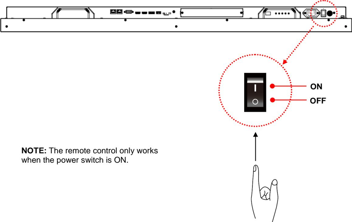
**NOTE:** The remote control only works when the power switch is ON.
