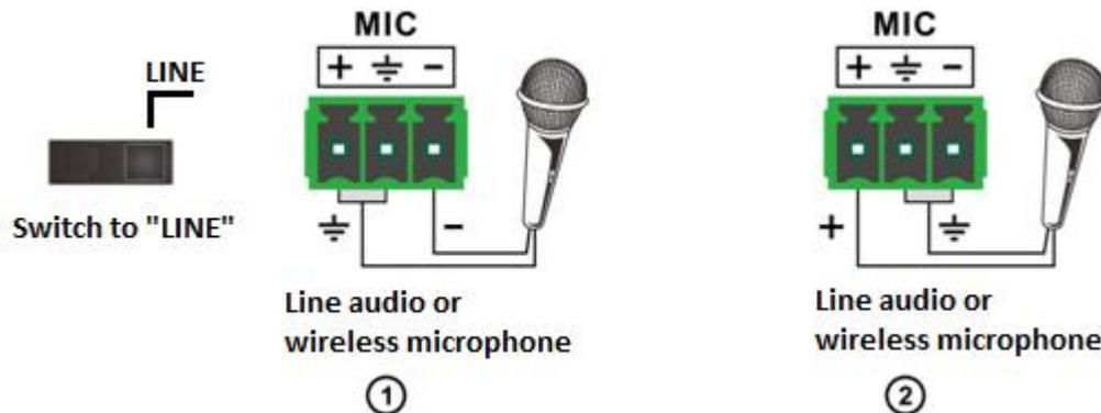
2) Balanced connection: “+” connects to positive, “-” connects to negative and
