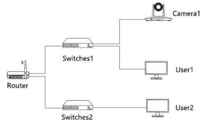
Please refer to the above diagram, user1 and user 2 are in the same router, they are considered as in the same LAN, connect the camera to the same LAN as where the PC is, and refer to below instructions as how to use the application software, then the camera can be found and connected from the online device list.
