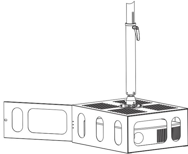
**Note:** When the projector light is on the left, the projector should be installed in the opposite direction.
