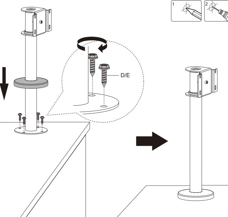
The VESA plate should be installed in the right direction as shown.
