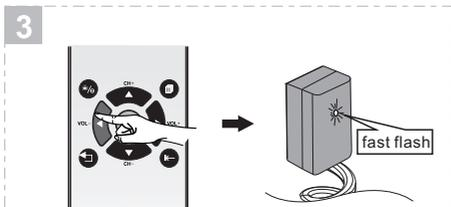
Target your TV remote control at the IR receiver, and press a button that is correspondent with the function of "OK" button. Then, the buzzer beeps three times, and the IR receiver flashes quickly.
