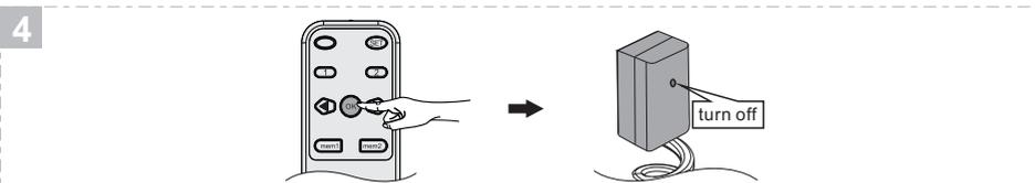
Press the "OK" button. The buzzer will beeps 4 times, and the IR receiver turn off. The duplication is successful.
