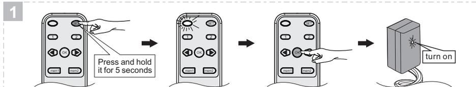
Press and hold the "SET" button for 3s. When the LED indicator on the remote control lightens continuously, press the "OK" button. The buzzer will beep once. After the IR receiver lightens, the system enters learning mode.
