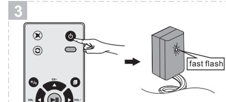
Target your TV remote control at the IR receiver, and press a button that is correspondent with the function of "1" button. Then, the buzzer beeps three times, and the IR receiver flashes quickly.
