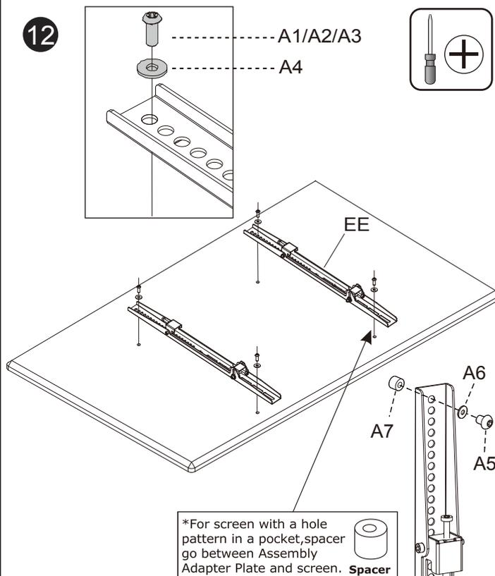
\*For screen with a hole pattern in a pocket, spacer go between Assembly Adapter Plate and screen. **Spacer**
