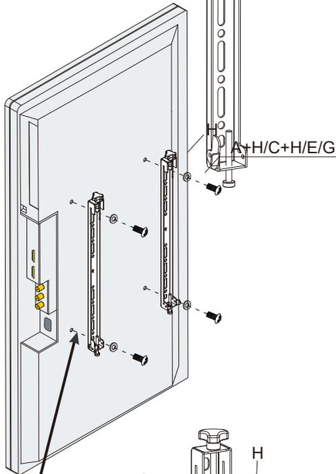
\*For screen with a hole pattern in a pocket, spacer go between Assembly Adapter Plate and screen.
