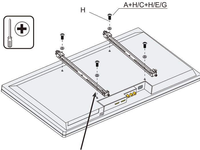
\*For screen with a hole pattern in a pocket, spacer go between Assembly Adapter Plate and screen.
