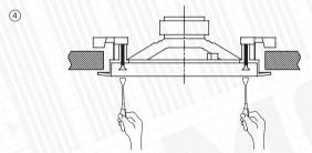
Carefully push speaker in the cut hole and fix the loudspeaker with mounting screws. Mount the grill on the loudspeaker.
