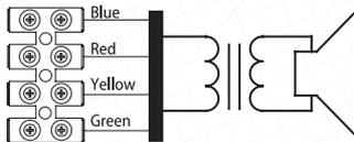
Connect speaker to signal line via block terminal.
