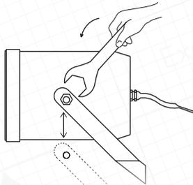
Remove mounting bracket from loudspeaker.
