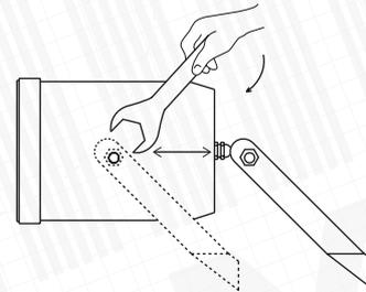
Place loudspeaker in mounting bracket and set rotation angle.
