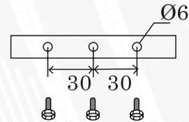
Fix mounting bracket on the flat surface.
