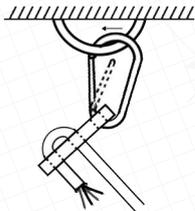
Mount the eye bolt in the ceilings and fix spring hook on it.
