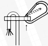
Place the spring hook in the hole of cable clip.
