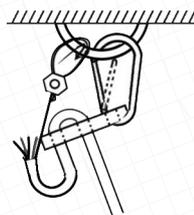
Make the loop in the end of the wire rope and fix the clamp.
