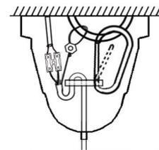
Lift the dome to hide the mounting hardware. Gently tighten up the screw in a dome to prevent slip.
