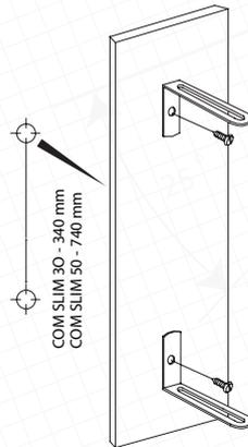
Fix mounting bracket on solid surface (recommended distance between brackets center holes 340 mm for COM SLIM 30 and 740 mm for COM SLIM 50)
