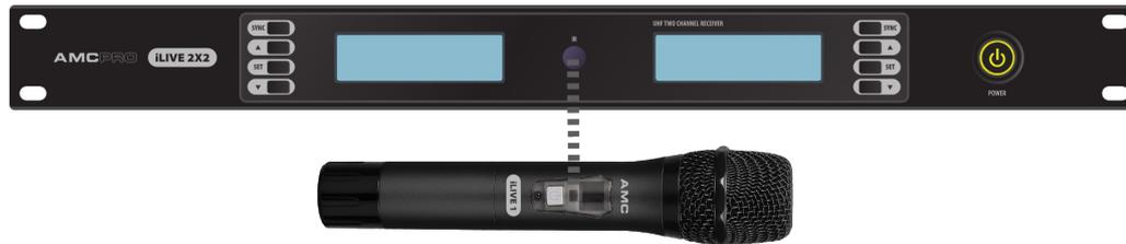
**IMPORTANT:** During synchronization IR receiver and IR transmitter should be directed to each other.
