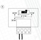
4. Use the power switch to select the required power.
