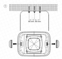
1. Drill three holes in the wall and use reliable screws suitable for your wall type. The distance between the holes should be 80 mm. Fix mounting brackets on the wall. Then fix the horn loudspeaker on the bracket. Tighten the screws and put on the screw covers.
