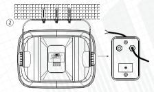
2. Remove the cover and insert the cable throw the PG connector.
