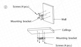
2. Fix subwoofer bracket on solid surface. Please use the proper screws for your wall or ceiling type.
