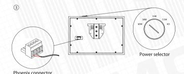
3. Connect audio cable to phoenix connector and set up right tranformers power. Please take attention to polarity. 4  $\Omega$  power tap should be used with low impedance amplifier.
