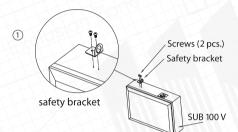
If needed fix safety bracket on the subwoofer by using two wood screws. To ensure safety, fix subwoofer by using safety rope to the reliable base. Safety rope is not supplied and should be purchased separately.
