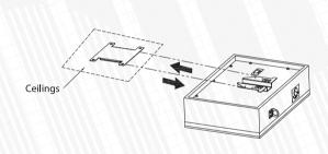
4. Put subwoofer on the mounting bracket and push it down till click sound appears. Please ensure that subwoofer is mounted reliable. Lift subwoofer strongly in order to release the lock and move it from mounting bracket.
