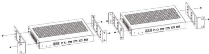
**Step 2:** Use screws to fix two 1U V2 rack brackets together, as shown in the figure below:
