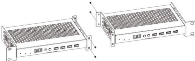
**Step 3:** Fasten screws between two 1U V2 rack brackets, so that two products are mounted in a 1U V2 rack, as shown in the figure below:
