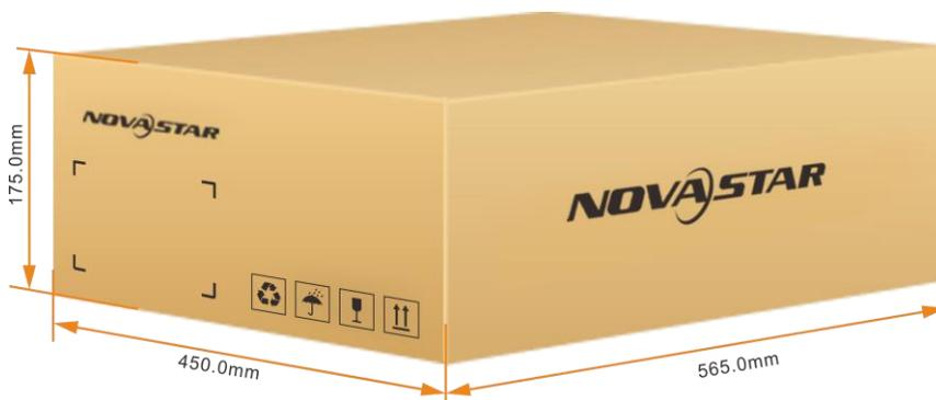
Tolerance:  $\pm 5$  Unit: mm
