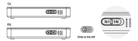
Multiple transmitters (TX) can wirelessly stream to a single receiver (RX). Both the TX and RX switch buttons must be set to **N-to-1 mode** for proper operation.
